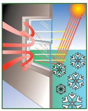
Low-E glass is engineered to provide year round comfort, keeping your home cooler in summer by keeping out unwanted solar heat and warmer in the winter by keeping furnace heat inside.
